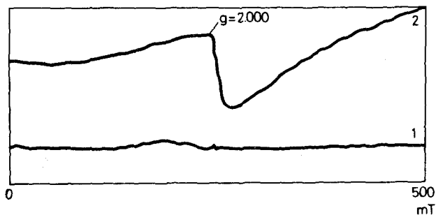
Fig. 4 ESR spectra of chalcopyrite-pyrite mixtures. 1: non-activated sample; 2: mechanically activated sample, t_M = 1 hour
